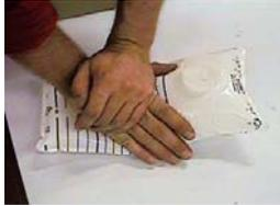
1. Blow up the bag and check that the welding is intact after that the bag has explored.
