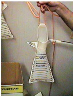
7. Keep the volume of water in the unit; hang up the unit in its funnels handle under a period of 48 h. Thereafter check the handle of the funnel and the welded area of the bags funnel receiver.
